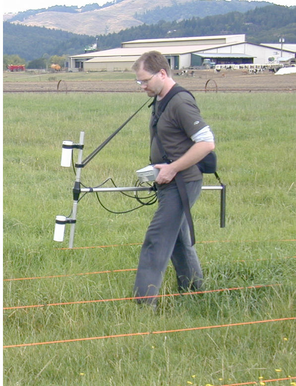
Figure 1. Cesium magnetometer in vertical gradient mode and operator walking a typical survey transect.
